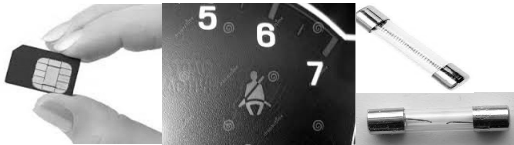
Figure 1. Three Types of Poka yoke (a) Control (b) Warning (c) Shutdown
